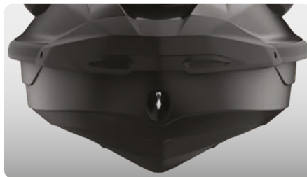
GTI™ Hull This moderate V-shaped hull guarantees a stable, enjoyable ride in variable water conditions. Confident, predictable handling but incredibly playful when you want it to be.
