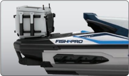
Rear Deck Extension with LinQ attachment system Adds 11.5 inches to the back of the watercraft to increase stability, space, and storage capability.
