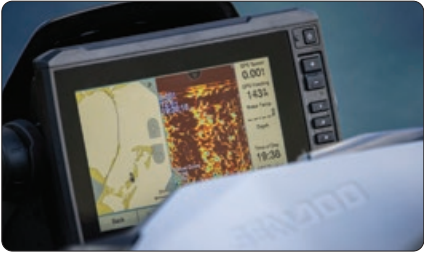
Garmin 7 in. GPS & Fish Finder A top-of-the-line navigation, charting and fish-finding system using an in-hull transducer and mid-CHIRP sonar.
